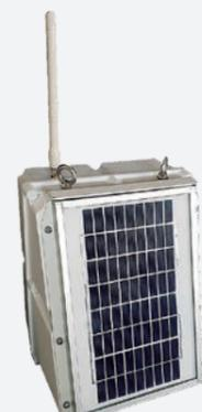
IoT terminal for water level monitoring
